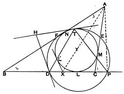
Let L, M, N be the points of contact of the inscribed circle with the sides of the triangle. Let D be the middle point of BC, and P the foot of the perpendicular from A. Let the line joining A to the centre of the inscribed circle cut BC in X, and let XL' be the other tangent drawn from X to this circle. Join DL', and let it cut the inscribed circle in T. Then T is a point on the nine-point circle, and the two circles will touch at T.
